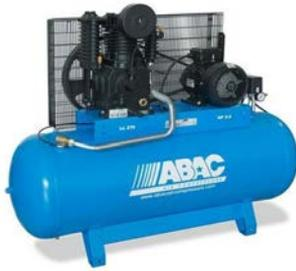
Piston compressors with fully cast iron blocks: a reliable and robust range, built with top quality components. The pumps are running at a low speed, to guarantee lower noise levels, lower operating temperatures and extended lifetimes, but they still guarantee a great performance, and they are perfectly suitable for the more demanding and intensive applications.
