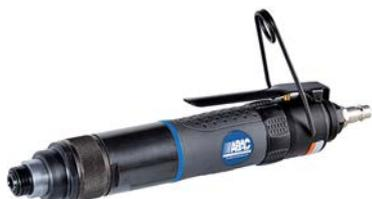
Compact screwdriver for professional use in wood- and metalworking industries. Anti-slip, ergonomic handle. Extremely low noise due to exhaust air silencer. Stemless torque adjustment on the outer adjusting ring allows for flexible working. Suitable for hanging on balancers.
