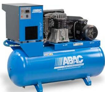
This two stage belt drive compressor is a 5.5 HP static compressor mounted on a 270 litre receiver, suitable for a workshop where three phase is available. This compressor is the perfect choice for medium workshops. With the addition of a refrigerant air dryer it becomes a complete air station producing dry compressed air providing better quality air for air tools and paint spraying.
