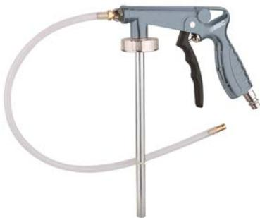
Spraying gun for car application such as anti noise treatment or body-cavity seal. Suitable for standard 1l cans with 40mm thread. Injection probe with four side spray orifice for use in tighten places of car body. Multi purpose spray gun.
