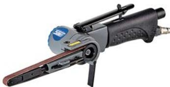
Compact belt sander for professional use in wood and metalworking industries and car workshops. Exhaust air guide towards the rear prevents swarf dispersion. Actuating lever with trigger safety device. Automatic belt tensioner for easy abrasive belt changing.
