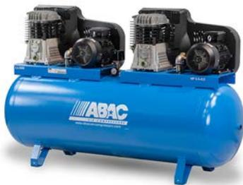
Our PRO tandem units are fitted with two double stage pump units delivering high outputs. As everything gets larger and heavier we have mounted these units on heavy duty air receivers and given them a large 500 litre storage volume to ensure correct operation. Metal guards and star delta starter assembly complete this heavy duty compressor designed for more demanding operations.
