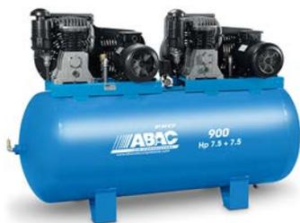
Our B6000 900 LT high flow tandem air compressor units are ideal for those users who are looking for high volume output from a compact footprint. Two identical compressor / motor units mounted on a single air receiver they can operate together using the same pressure switch or with the addition of a second pressure switch they can be configured as duty / standby units.
