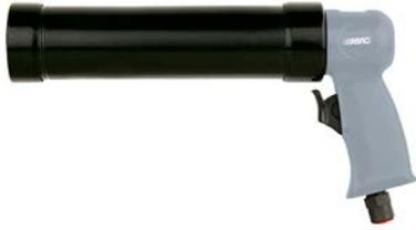
Cartridge gun for standard 310ml plastic cartridges. Multiple use can be used for silicon and adhesives. Quick pressure release by pushing the venting valve. Fast and easy sealing without manual efforts.
