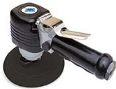
Compact orbital sander for several DIY and semi professional sanding applications, especial for large surfaces. Quick work progress due to the high revolution and 5mm stroke. Sanding pad with touch fastener for standard 150 mm without holes. Rubber handle cover isolates, reduces vibrations and provides more grip.
