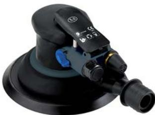
Universal orbital sander with 5mm stroke. Fatigue-free grinding thanks to reduced vibrations. Unlimited view of the workpiece with narrow collar. Particularly low air consumption. Suitable for standard 150mm, 15-hole, 8-hole and 6-hole sanding paper.
