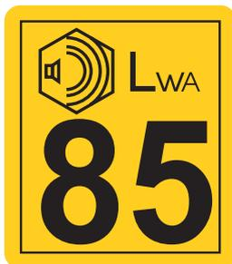
Compressor Label Sound Values: In accordance with CEE regulations, it is mandatory for the sound power level (LWA) to be clearly displayed on all air compressors.
