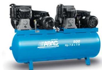
Our PRO tandem units are fitted with our two double stage pump units delivering high outputs. As everything gets larger and heavier we have mounted these units on heavy duty air receivers and given them a large 500 litre storage volume to ensure correct operation. Metal guards and star delta starter assembly complete this heavy duty compressor designed for more demanding operations.
