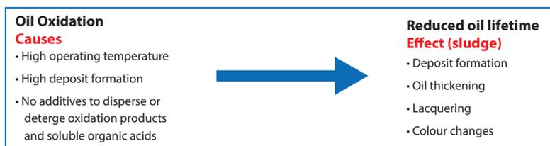
Anti-oxidant additives delay the oxidising process, deposit and acid formation to extend oil lifetime and protect equipment during stand-still period.
