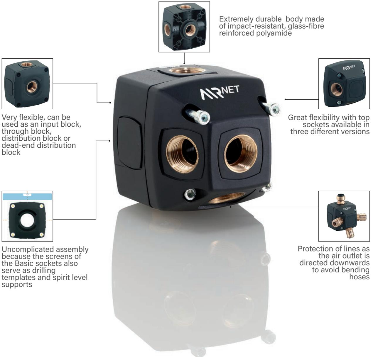
Install perfect compressed air outlets in the pipe system for each workplace. Versatile pipe sockets are fully compatible with the AIRnet pipe system and various attachment parts and can be extended by fitting additional outlet components.
