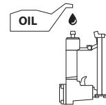
Wipe off any excess oil in the outlet. Excess oil may damage the O-ring seals of the tool. If a lubrication system is used, manual lubrication through the air inlet will not be necessary on a daily basis.
