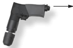
**5.2** Add a few drops of tool oil to the air inlet. Position the tool with the air inlet connector facing upwards and place a drop of tool oil inside the air inlet. Do not use cleaning oil or additives. Put the tool into operation briefly after adding the oil (2).
