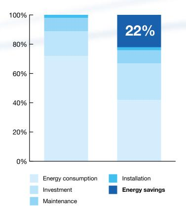
Air consumption within the network is not constant over time. A variable speed compressor lowers the speed of the motor according to the compressed air consumption. In this way, you can achieve major electricity savings.
